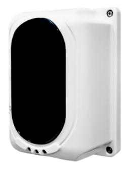
Infrared fire barrier - Range up to 100 metres - Display and laser pointer for easy installation - Opening of 14 meters (7 on each side) - Adjustable sensitivity - Certificate EN54-12:2015
