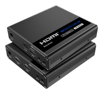
HDMI active Extender - Transmitter and receiver - Range 60 m - Over cable UTP Cat 6 - Up to 4K - Power supply DC 5 V
