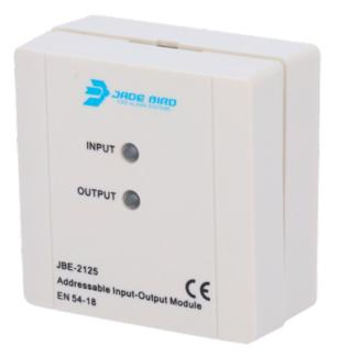
Jade Bird analog module - 1 Output with confirmation input - Powered by loop - Conductor cable up to 2.5mm2 - REOL of 10 k? (supplied) - Certified EN 54-18
