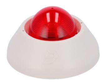
Jade Bird analog siren - High power output 100 dB(A) @ 1m - Requires auxiliary power supply of 24 VDC - Base not included - Indoor installation - Certified EN 54-3
