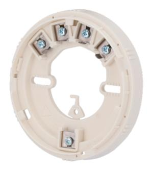
Jade Bird connection base - Basis of 4 terminals - Connection without polarity - 4 terminals, 2 loop and 2 external power supply. - Compatible with all Jade Bird devices - Allows connection of remote indicators or pilots
