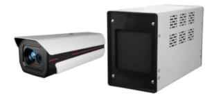
Precise Body Temperature Measurement System - Remote body temperature measurement - Thermographic Camera: 384x288 Vox | 10mm Lens - Blackbody for automatic calibration and ensuring accuracy - High Accuracy ±0.3°C - Monitoring and management software
