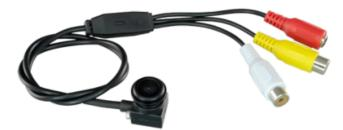
Ultraminiature camera - 1/4" Aptina© 960H CMOS MT9V139 - Extension cable 0.5 metres - Wide angle lens 1.8 mm - 0.1 Lux / F2.0 - 14 x 14 x 20 mm, 27 g
