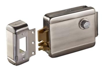
Electromechanical surface lock - Fail Safe (NC) opening mode - Applicable for firefighting systems - LED status indicator - Programmable self-closing - Right-hand opening outwards
