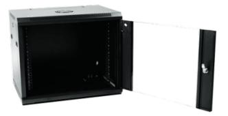
Rack cabinet for wall - Up to 9U rack of 19" - Up to 100 kg load - With ventilation and cable passage - Depth 600 mm - Supplied disassembled
