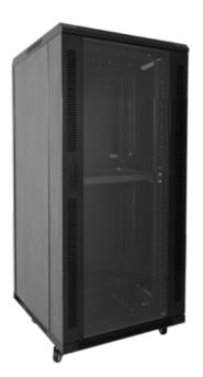
Rack floor cabinet - Up to 18U rack of 19" - Up to 800 kg load - With ventilation and cable passage - 2 fans, 2 trays and terminal strip 6 sockets - Supplied disassembled
