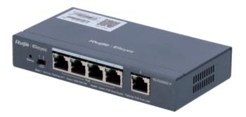
Reyee Manageable Cloud PoE Switch - 4 802.3af/at PoE port(s) + 1 Up-link port(s) - 4 RJ45 10/100/1000Mbps + 1 RJ45 10/100/1000Mbps - 30W per port 802.3af/at / Maximum 54W - VLAN/Port Isolation/Loop Detection - Port Speed Limit
