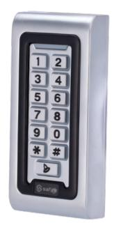
Standalone access control - EM card and PIN access - Relay, pushbutton and buzzer outputs - Wiegand 26 - Time control - Suitable for exterior IP68
