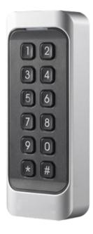
Access reader for frames - EM card and PIN access - LED and acoustic indicator - Wiegand 26/34 | RS485 - Compatible with Safire - Suitable for exterior IP65
