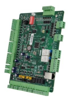
Biometric access control panel - Access by fingerprint, facial, card or password - TCP/IP | eHome | ISAPI | OSDP communication - 4 Wiegand inputs 26 y 4 RS485 - Relay output for two doors - Safire Control Center-software
