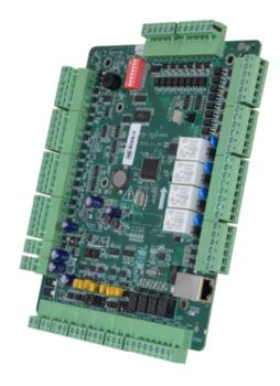
Biometric access control panel - Access by fingerprint, facial, card or password - TCP/IP | eHome | ISAPI | OSDP communication - 4 Wiegand inputs 26 y 8 RS485 - Relay output for four doors - Safire Control Center-software
