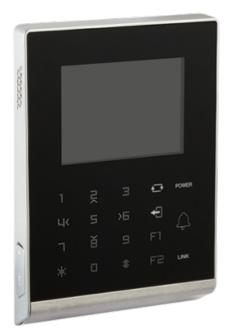
Access and Attendance control - EM card and keypad - 100.000 users / 300.000 registers - TCP/IP, USB, WiFi, Wiegand and Relay - Integrated controller - Safire Control Center-software
