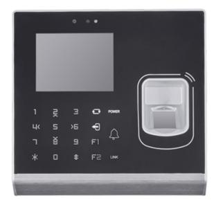
Access and Attendance control - Fingerprints, EM card and keypad - 3.000 recordings / 100.000 records - TCP/IP, USB, WiFi, Wiegand and Relay - Integrated controller - Safire Control Centersoftware
