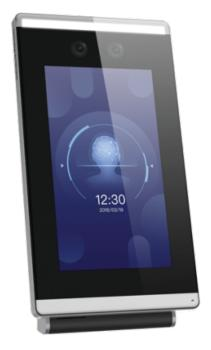
Access and Attendance control - Facial recognition and passwords - 20.000 faces / 100.000 records - TCP/IP, RS485, Wiegand, USB and WiFi - Door sensor, push button and relay - Software Safire Control Center AC
