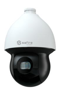
Safire Smart - IP PTZ gamma camera I1 Artificial Intelligence - Resolution 4 Megapixel (2560x1440) - Optical zoom 40X | IR 350m - Autotracking, human and vehicle | Alarms - Waterproofing IP67 & IK10 | PoE+ (IEEE802.3at)
