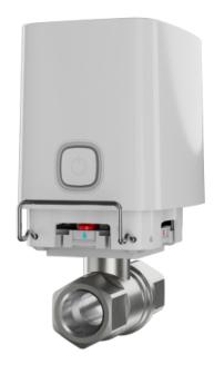
Solenoid water shutoff valve - Bonomi Valve of 1/2" (DN 15)) - Compatible with hot and cold water pipes - Valve closing in less than 5 seconds - Supports automation scenarios - Power 4 batteries CR123A or at 7,5~14 VDC
