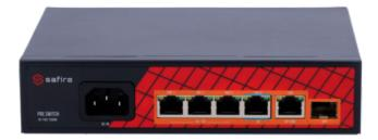
Safire Switch Hi-PoE - 4 PoE ports + 1 Uplink RJ45 + 1 SFP Uplink - Gigabit port speed 10/100/1000Mbps - 3 PoE+ ports 30W + 1 Hi-PoE port 60W - PoE Watchdog - Up to 65W Total PoE Power
