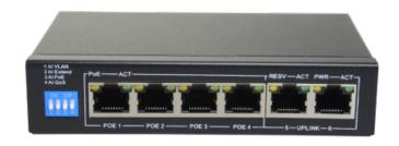
PoE Switch - 4 PoE port(s) + 2 Up-link port(s) - Speed up to 100 Mbps on all ports - Up to 60W in total for all ports - Bandwidth 1.2 Gbps - Standard IEEE802.3af (PoE) / at (PoE+)
