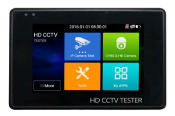
Multifunctional wrist held CCTV tester - Supports HDTVI, HDCVI, AHD, CVBS and IP cameras - Tester resolution up to 4K - Colour LCD display 4" - 2400mA Built-in Battery - Easy to use
