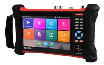
Multifunctional CCTV Tester - Supports HDTVI, HDCVI, AHD, CVBS and IP cameras (4K) - Colour LCD display 7" - Test of video, audio, UTP and TDR cables - Built-in battery 5000 mAh - WiFi connection / Digital multimeter
