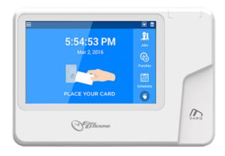
Time & Attendance control - EM RFID cards and keypad - 1.000 users / 1.000.000 registers - WiFi, TCP/IP, USB and Wiegand and PoE - 5.0" Touch screen - EasyClocking Cloud Software not inc.
