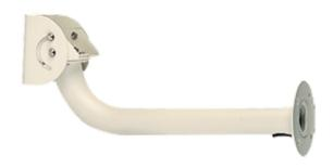
Front bracket for housing - Compatible with HS250W - 170 (H) x 85 (W) x 305 (D) - Maximum load 15 Kg - Aluminum / Ivory colour - Horizontal 360° / vertical 85° rotation
