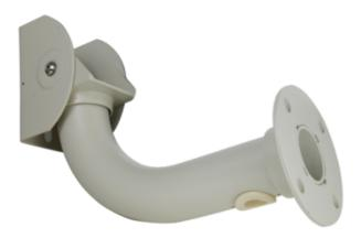
Lateral bracket for casings - Compatible with HS250W - 170 (H) x 85 (W) x 170 (D) - Maximum load 15 Kg - Aluminum / Ivory colour - Horizontal 360° / vertical 85° rotation
