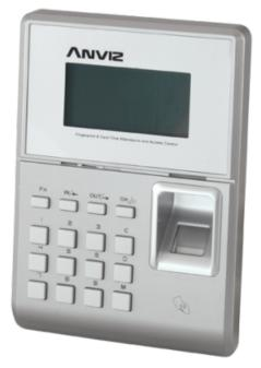
Time & Attendance and Access control - Fingerprints, RFID Card and keypad - 2000 recordings / 50000 records - TCP/IP, USB, USB Flash, Wiegand, Relay - 8 Time & Attendance control modes - Integrated controller
