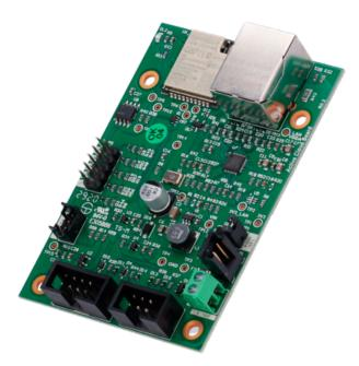
URFOG - LAN board for Modular range - Allows you to connect the control panels to the cloud - Allows remote monitoring - Real-time machine vision - Installation cables included
