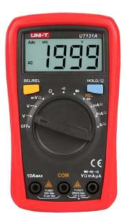
LCD handheld digital multimeter - DC and AC voltage measurement up to 250V - DC and AC current measurement up to 10A - Auto range of measurement - Resistance and capacitance measurement - Buzzer for continuity test
