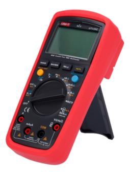
Digital multimeter with True RMS function - DC and AC voltage measurement up to 600V - DC and AC current measurement up to 10A - Resistance, Capacitance and Frequency Measurement - Temperature measurement - Buzzer for continuity test
