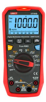
Digital multimeter CAT III - LED display up to 6000 accounts - DC and AC measurement up to 1000V and 20A - PC connection - High AC accuracy with True RMS function - Measures resistance, capacitance and temperature
