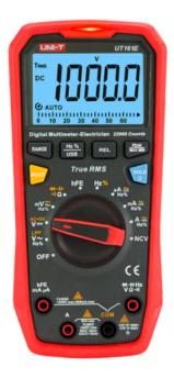
Digital multimeter CAT III - LED display up to 22000 accounts - DC and AC measurement up to 1000V and 20A - PC connection - High AC accuracy with True RMS function - Measurement of resistance, capacitance and hFE
