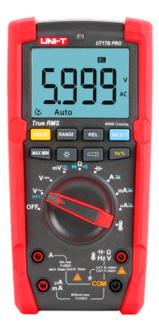
True RMS digital multimeter - DC and AC voltage measurement up to 1000V - DC and AC current measurement up to 10A - Resistance and capacitance measurement - Temperature measurement - Buzzer for continuity test | Diodes test
