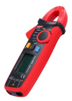
Mini clamp ammeter - DC and AC measurement up to 600V and 100A - Measures resistance and capacitance - Auto Range | Diode Test - True RMS | Continuity Buzzer | NVC - Clamp opening of 17mm
