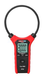
Flexible current clamp 10" - LCD display of up to 3000 counts - Current measurement in AC up to 3000A - High AC accuracy with True RMS function - Degree of protection IP54 | 2m drop test [%VAR%] - Automatic shutdown
