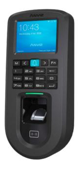
ANVIZ autonomous biometric reader - Fingerprints, RFID and keypad - 3000 recordings / 100000 records - TCP/IP, WiFi, RS485, miniUSB, Wiegand 26 - Integrated controller / PoE - Anviz CrossChex Software
