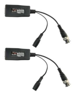
SAFIRE UTP passive transceiver - 4N1 (HDTVI, HDCVI, AHD and CVBS) - 1 video channel and power supply - Connector RJ45, BNC and Jack - Range: 190 ~ 440 m - 2 units
