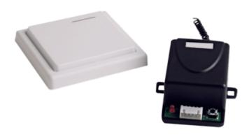
Wireless relay - Includes wireless push button - Operation NO/NC - Frequency 433 MHz - Up to 50 meters of transmission - Easy installation
