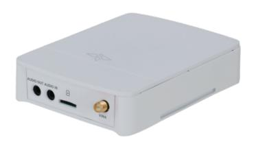
Main Box for X-Security mini cameras - 4 Megapixel (2592x1944) - Has to be combined with a lens - Capacity for 3 streams - Compression H.265+/H.265/H.264+/H.264 - PoE IEEE802.3af
