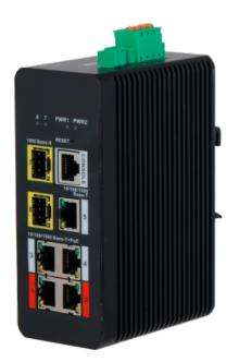
X-Security PoE Switch DIN Rail - 4 PoE ports RJ45 + 1 port RJ45 + 2 SFP - Speed 10/100/1000Mbps - 90W ports 1-2 / 30W ports 3-4 / Maximum 120W - PoE/PoE+/Hi-PoE / Up to 250m / PoE Watchdog - VLAN/STP/RSTP/ERPS/LACP/StaticLAG/IGMP Snooping
