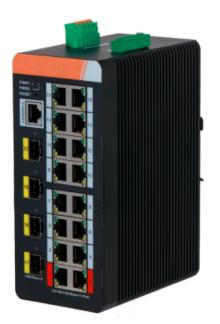
X-Security PoE Switch DIN Rail - 16 PoE RJ45 + 4 SFP ports - Speed 10/100/1000Mbps - 90W ports 1-2 / 30W ports 3-8 / Maximum 120W - PoE/PoE+/Hi-PoE / Up to 250m / PoE Watchdog - VLAN/STP/RSTP/ERPS/LACP/StaticLAG/IGMP Snooping
