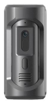
Video intercom IP - Camera 2Mpx wide-angle with WDR - Bidirectional audio - Mobile App for remote monitoring - IK10 protection anti-vandal - Surface mounting | PoE
