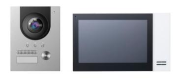
Video-intercom kit - IP and PoE Technology - Includes panel and monitor - PoE switch and bracket inc. - Mobile App with P2P - Surface mounting
