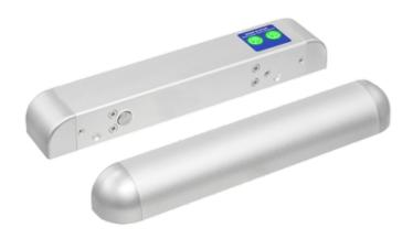
Electric security lock - Fail Safe (NC) opening mode - Holding force 1000 kg | Door sensor - LED status indicator - Programmable self-closing - Selectable opening time
