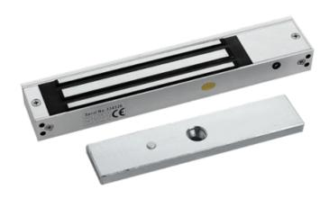
Electromagnetic door lock - For single doors - Fail Safe mode - Retention force 180 Kg - Power supply DC 12 V - Different compatible profiles
