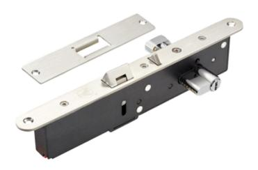
Electromechanical safety lock - Fail Secure and Fail Safe opening mode - Holding force 500 kg | Door sensor - Bidirectional opening - Stainless steel SUS304 - European cylinder included with keys
