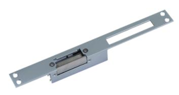
Electrical door openers - For single doors - Fail Safe (NC) opening mode - Holding force 500 kg - Power supply DC 12V - Recessed mounting | Socket
