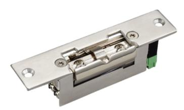
Electrical door openers - For single door | Adjustable latch - Opening mode Fail Secure (NO) | Gate signal - Holding force 300 kg - Power supply DC 12V - Flush mounting
