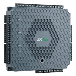
PoE biometric access controller - Access by fingerprint, card or password - TCP/IP | Connection to slave controller - 4 readers by Wiegand | 8 readers by OSDP - Relay output for 4 doors - Embedded ATLAS Series software and mobile app
